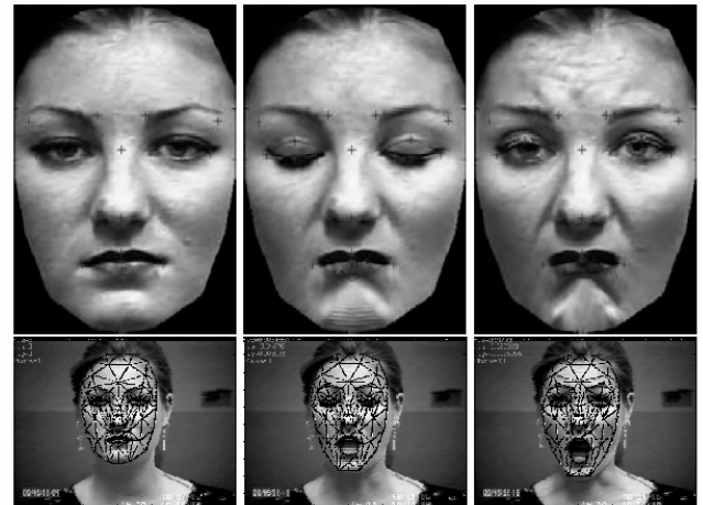
Figure 5. Example of posture and morphing estimation and frontal view normalization on Cohn-Kanade DataBase.
