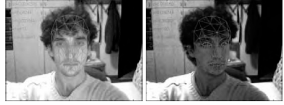
Figure 4. Tracking 3D with global illumination robustness technique.
