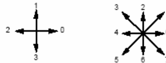
Figure 3. Different directions of Freeman coding
