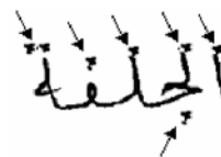
Figure 4a: Projection of the segmentation assumptions in the event of overlapping ▴: Points defined in the vertical optimums
