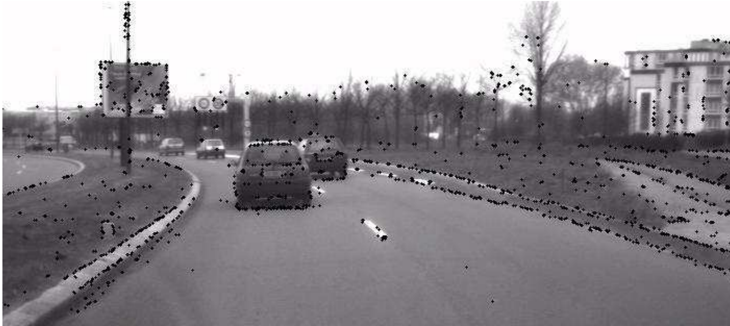
Real-time processing on a highway. The flies (black dots) concentrate on contrasted road edges and other cars.
